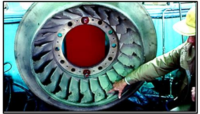
Cavitation erosion on old runner.
