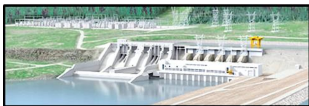
Site C project layout. Spillway on left.
