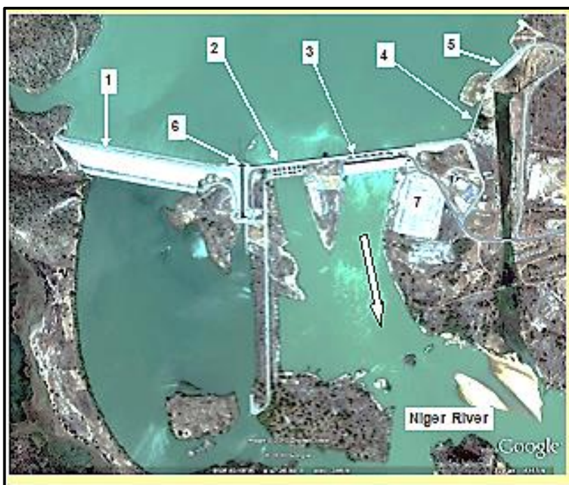
Jebba development. 1. Dam. 2. Spillway. 3. Powerhouse. 4. Emergency weir spillway. 5. Side dam. 6. Navigation lock. 7. Substation.
