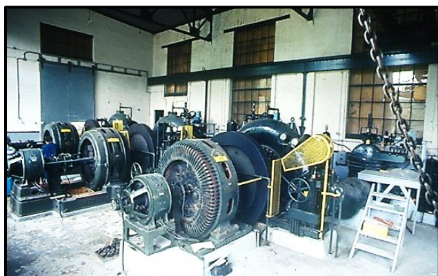
Powerhouse interior with three horizontal turbines.
