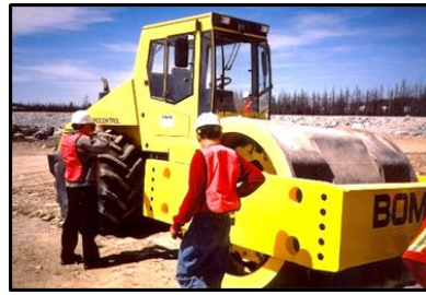
25 Ton Bomag vibrating octagonal roller compactor.
