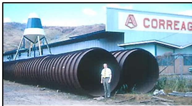
Inspecting penstock pipes fabricated locally in Panama.
