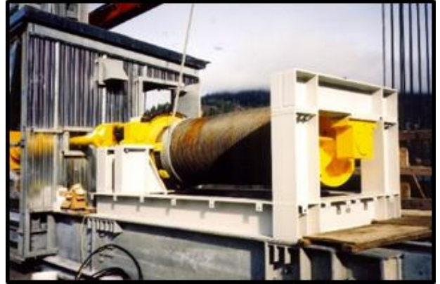
Hoist drum on deck, before installing housing with a slit in roof for the cable.
