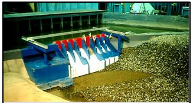
Model of main spillway. Note level of powerhouse draft tube deck.
