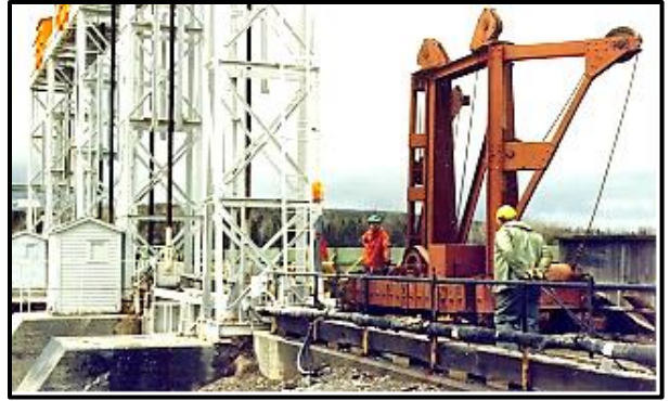
Travelling hoist for low level sluices.
