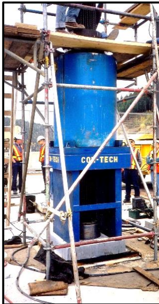
Jannox 550ton jack used to test anchor strands.
