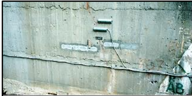
Crack instruments all wired to a recorder.
