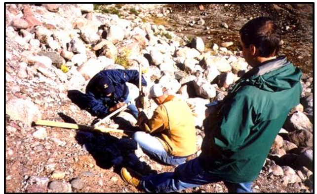
Steepest slope at 1.3:1 on GR-2.
