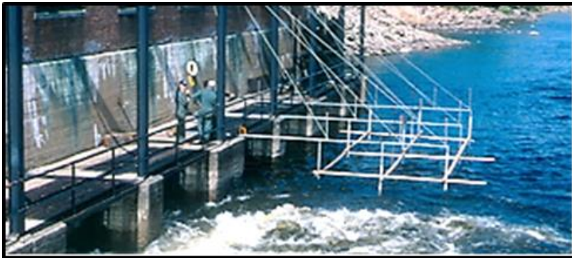
Array used to measure tailwater level. The instantaneous level for all 9 probes was averaged.
