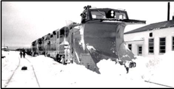
IOC supply train. 3 locomotives pushing snow plough.
