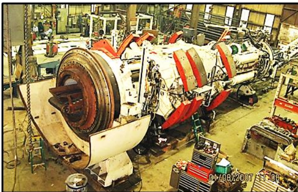
23 year old boring machine rehabilitation.
