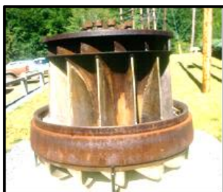
Very rare double-runner, smaller runner on top, vertical axis Francis unit, on display at the Hells Gate Dam.
