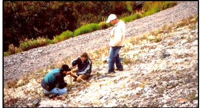
Measuring overly steep slope at GF-8, at 1.76:1.
