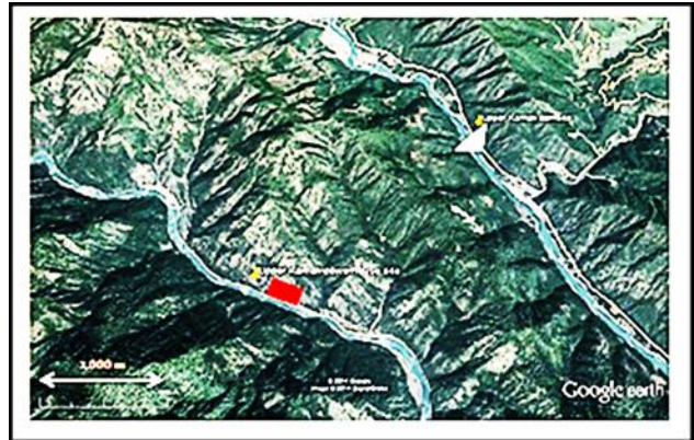
Google Earth view of site. Triangle is concrete dam, red oblong the powerhouse. Access tunnel and power tunnel between.
