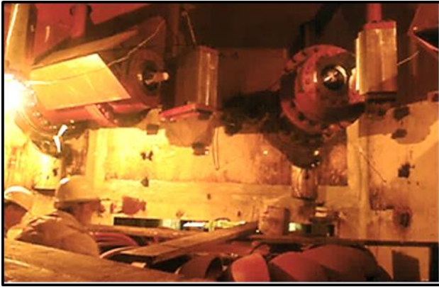
View of runner nozzles and jet deflectors.
