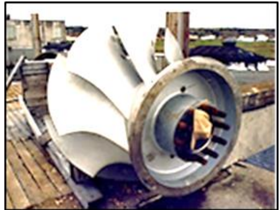
New mixed-flow propeller runner.
