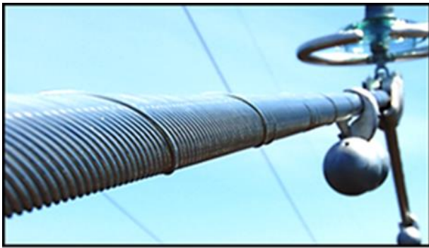
Defective transmission cable conductor with popped-out strand.
