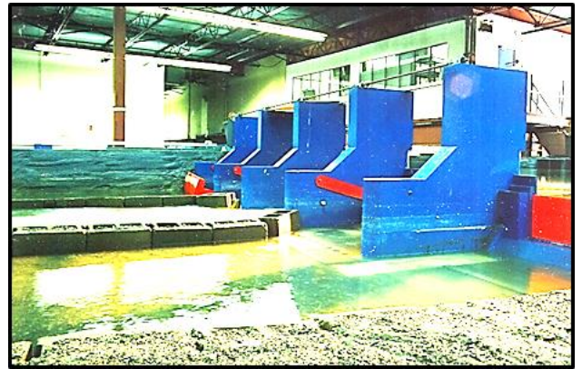
Hydraulic model of a spillway.
