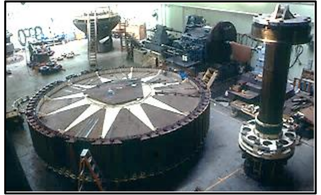
Motor-generator for pump-turbines.
