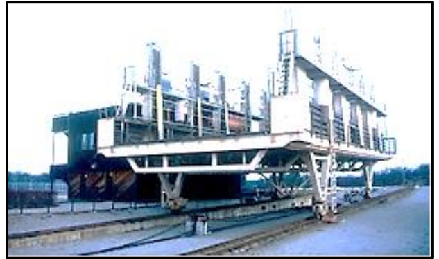
Rail transporter used to ferry boats over the dam.
