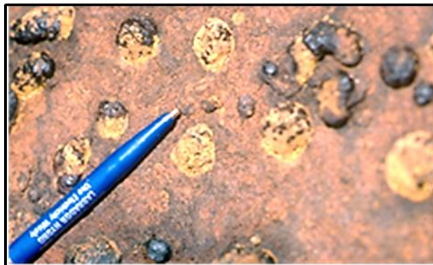
After wire brushing, erosion at weld joint.
