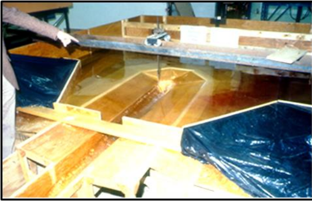
Bathtub spillway model at Memorial University.
