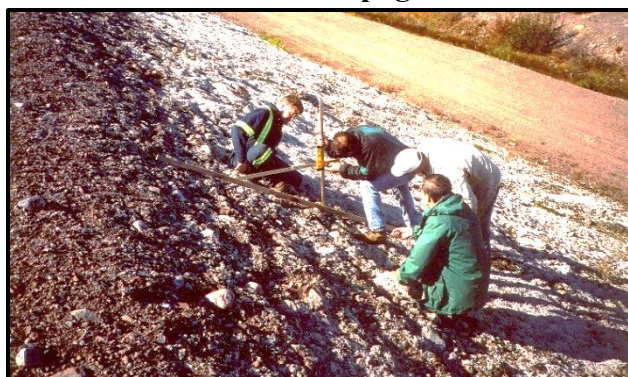
Measuring slope at GR-10 at 2.0 to 2.09:1.
