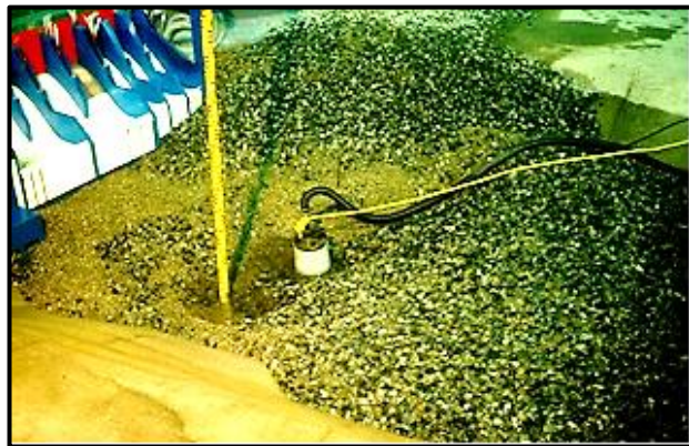
Measuring erosion depth after flood.
