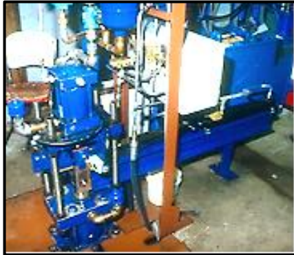
Relief valve controller. A complex combination of slider, pipes, valves, solenoids and pistons.
