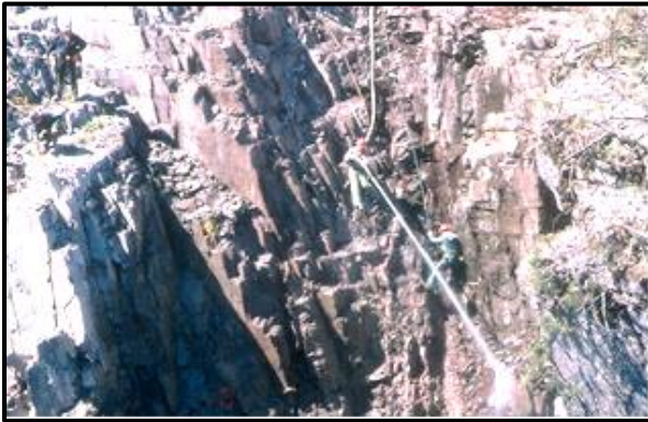
Removing overburden with water jet.
