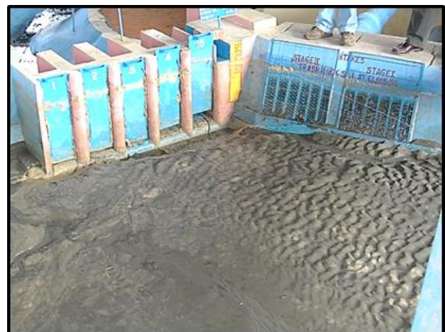
Intake racks almost covered with silt!
