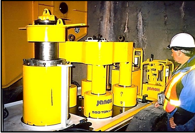
Jannox 550ton jack used to test anchor strands.
