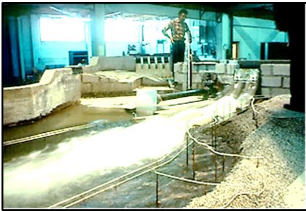
Hydraulic model of Dadin Kowa spillway.
