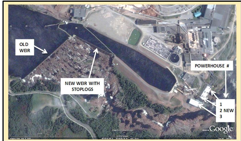
Grand Falls. Current layout showing canal, new intakes and powerhouse at location of the original powerhouse. Log boom across canal. Forebay gate structure retained to dewater canal if necessary.
