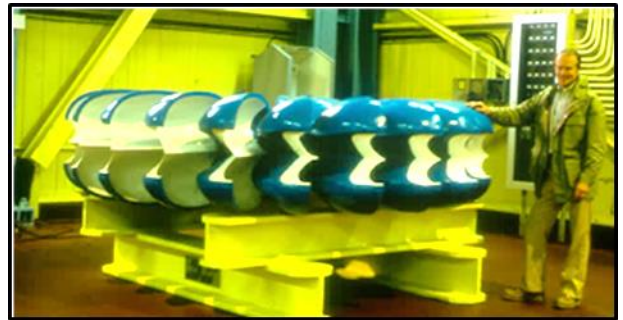
With spare runner – one of last by Fischer Castings.
