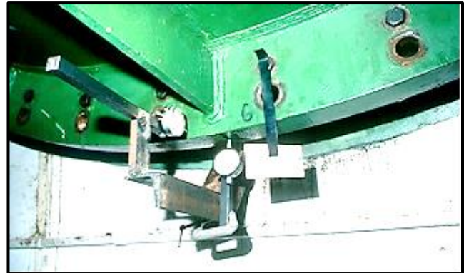
Dial gauges attached to underside of distributor ring.
